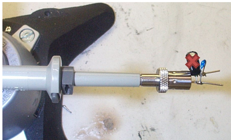
Figure 52 – Oscilloscope Probe with Probe Master ( www.probemaster.com ) 4987A BNC Adapter. (Modified with wires for ripple measurement, and one parallel decoupling capacitor added)
