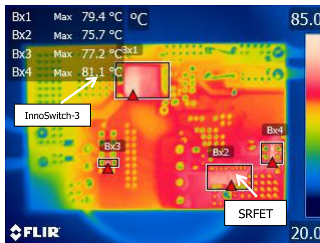
Figure 110 – 500 VDC 2.5 A Full Load. Temperature of InnoSwitch3-AQ: 79.4 °C. Temperature of SR FET: 75.7 °C. Ambient Temperature: 28.2 °C.
