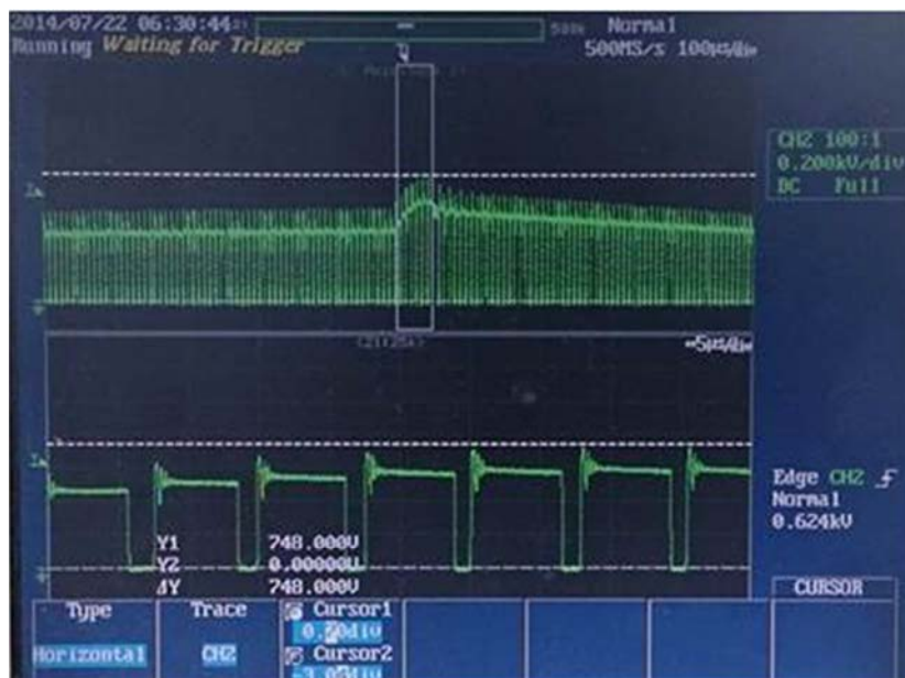
Figure 104 – Measured Peak Voltage: 748 V PK .
