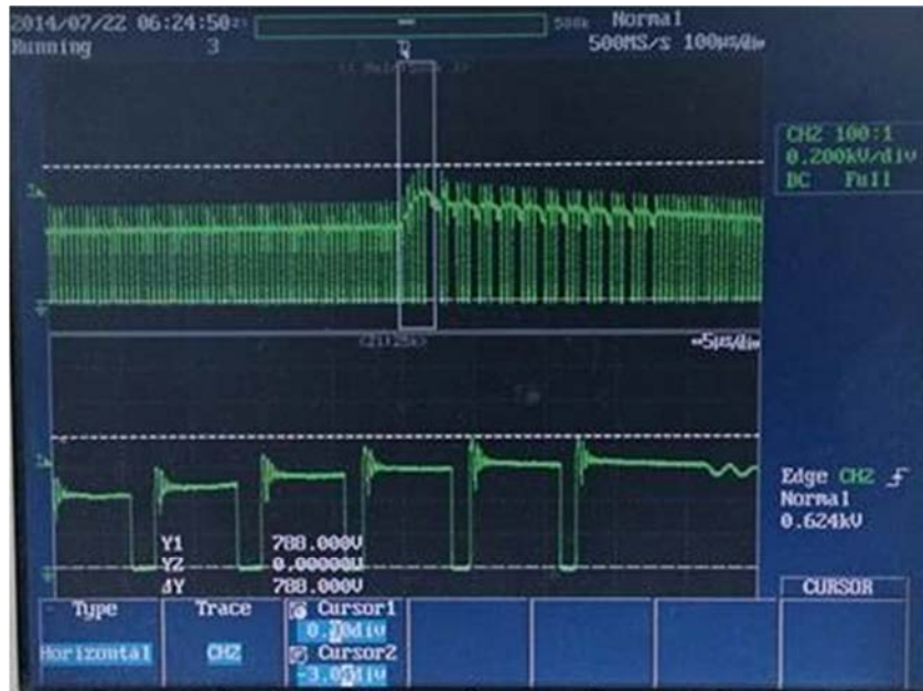
Figure 103 – Measured Peak Voltage: 788 V PK .
