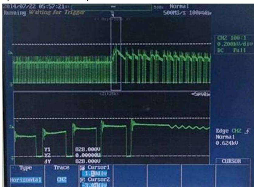
Figure 102 – Measured Peak Voltage: 828 V PK .
