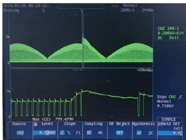
Figure 92 – 230 VAC, 50 Hz, +1000, 90°. Upper: V_{DRAIN} , 200 V / div. Lower: V_{DRAIN} , 200 V / div. (Zoomed). Measured Peak Voltage: 799.479 V_{PK} .
