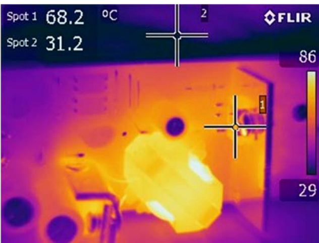
Figure 41 – 265 VAC, Full Load. Spot 1: LYT4325E. Spot 2: Ambient.
