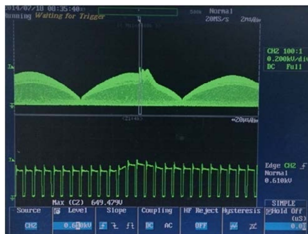
Figure 93 – 230 VAC, 50 Hz, -1000, 90°. Upper: V_{DRAIN} , 200 V / div. Lower: V_{DRAIN} , 200 V / div. (Zoomed). Measured Peak Voltage: 649.479 V_{PK} .
