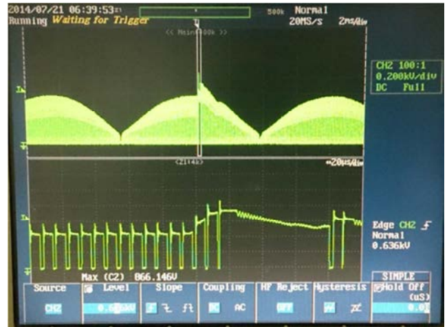
Figure 95 – 230 VAC, 50 Hz, -1000, 270°. Upper: V_{DRAIN} , 200 V / div. Lower: V_{DRAIN} , 200 V / div. (Zoomed). Measured Peak Voltage: 866.146 V_{PK} .
