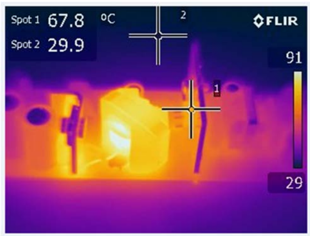
Figure 37 – 230 VAC, Full Load. Spot 1: LYT4325E. Spot 2: Ambient.
