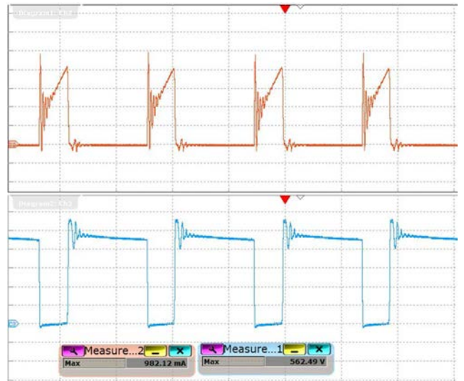
Figure 58 – 230 VAC, 50 Hz (zoomed version). Upper: I_{DRAIN} , 200 mA / div., 4 ms / div. Lower: V_{DRAIN} , 100 V / div., 4 ms / div. Measured V_{PK} at Normal Operation: 562.49 V_{PK} . Measured I_{PK} at Normal Operation: 982 mA_{PK} .
