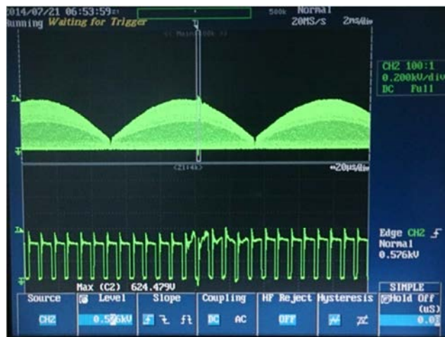
Figure 99 – 230 VAC, 50 Hz, -2500, 90°. Upper: V_{DRAIN} , 200 V / div. Lower: V_{DRAIN} , 200 V / div. (Zoomed). Measured Peak Voltage: 624.479 V_{PK} .
