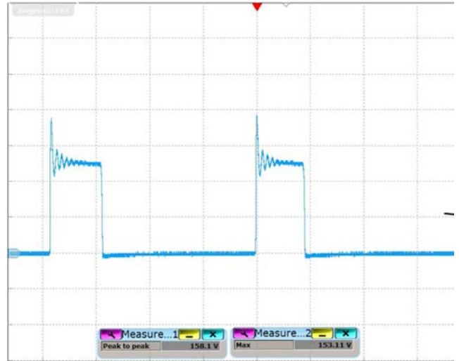
Figure 64 – 230 VAC, 50 Hz. V_{DIODE} , 40 V / div, 2 \mu s / div. Measured Diode V_{PK} : 153.11 V_{PK} .
