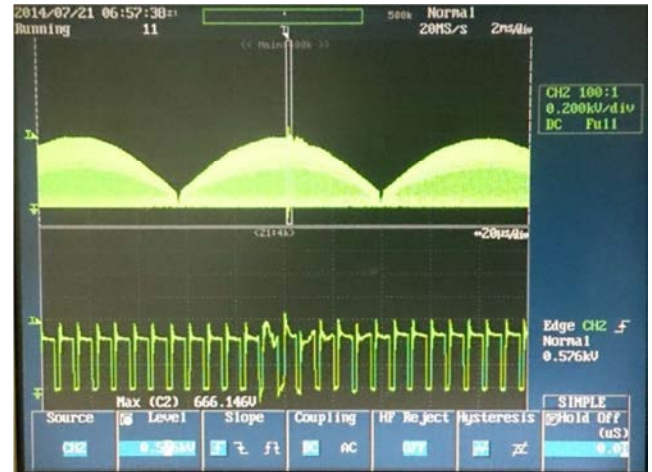
Figure 101 – 230 VAC, 50 Hz, -2500, 270°. Upper: V_{DRAIN} , 200 V / div. Lower: V_{DRAIN} , 200 V / div. (Zoomed). Measured Peak Voltage: 666.146 V_{PK} .
