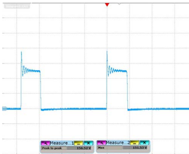
Figure 65 – 240 VAC, 50 Hz. V_{DIODE} , 40 V / div, 2 \mu s / div. Measured Diode V_{PK} : 151.53 V_{PK} .
