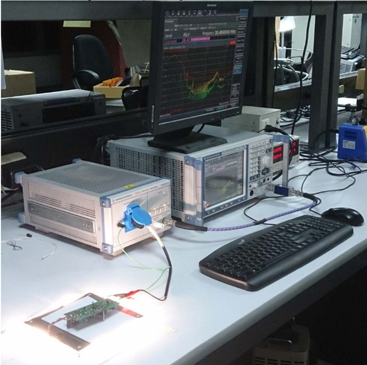
Figure 87 – Conducted EMI Test Set-up.
