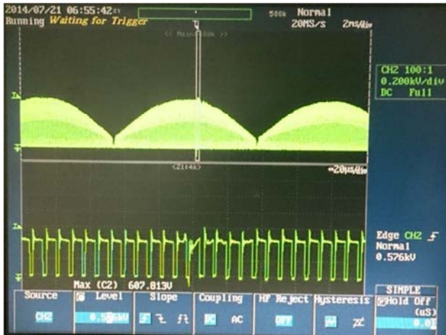
Figure 100 – 230 VAC, 50 Hz, +2500, 270°. Upper: V_{DRAIN} , 200 V / div. Lower: V_{DRAIN} , 200 V / div. (Zoomed). Measured Peak Voltage: 607.813 V_{PK} .
