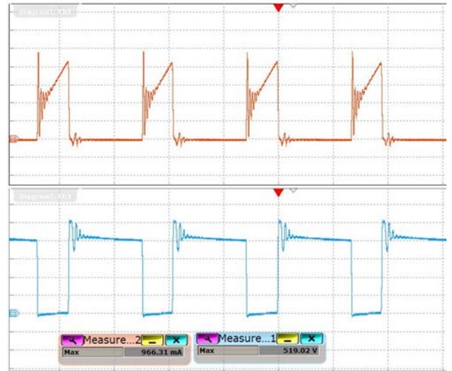
Figure 56 – 195 VAC, 50 Hz (Zoomed Version). Upper: I_{DRAIN} , 200 mA / div., 4 \mu s / div. Lower: V_{DRAIN} , 100 V / div., 4 \mu s / div. Measured V_{PK} at Normal Operation: 519 V_{PK} . Measured I_{PK} at Normal Operation: 966 mA_{PK} .
