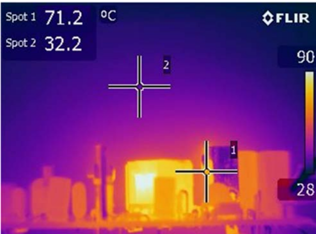
Figure 33 – 195 VAC, Full Load. Spot 1: LYT4325E. Spot 2: Ambient.
