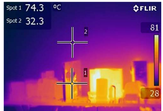
Figure 34 – 195 VAC, Full Load. Spot 1: Output Diode. Spot 2: Ambient.
