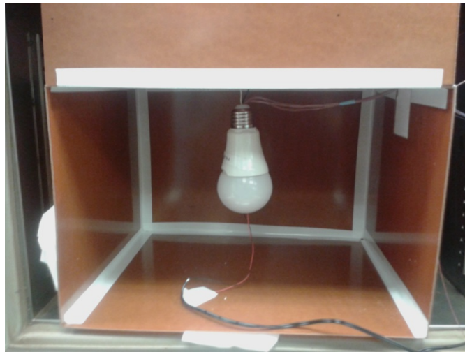
Figure 18 – Thermal Unit Thermocouple Measurement Set-up.
