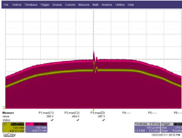
Figure 221 – Differential Ring Surge at 2500 V / 90°. Peak Drain Voltage Recorded is 464 V. Ch1: V_{BULK} ; 100 V / div. F1: V_{DRAIN} ; 100 V / div. Time Scale: 500 \mu s / div.
