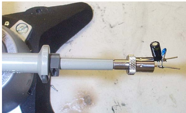
Figure 52 – Oscilloscope Probe with Probe Master ( www.probemaster.com ) 4987A BNC Adapter. (Modified with wires for ripple measurement, and two parallel decoupling capacitors added.)
