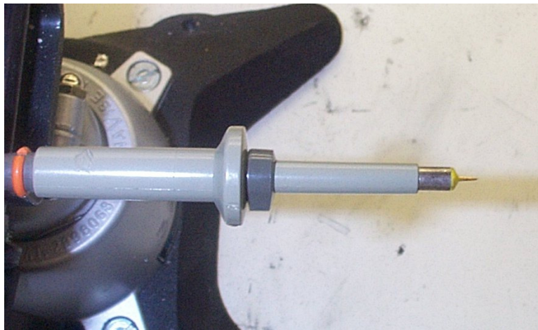
Figure 15 – Oscilloscope Probe Prepared for Ripple Measurement. (End Cap and Ground Lead Removed).
