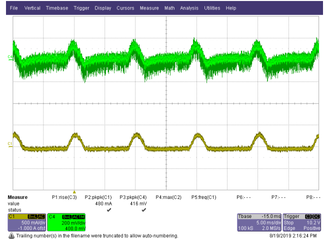
Figure 48 – Output Ripple, 180 VAC, 40 V CV Load. Green: V_{OUT} Ripple, 200 mV / div. Yellow: I_{OUT} Ripple, 500 mA, 5 ms / div.
