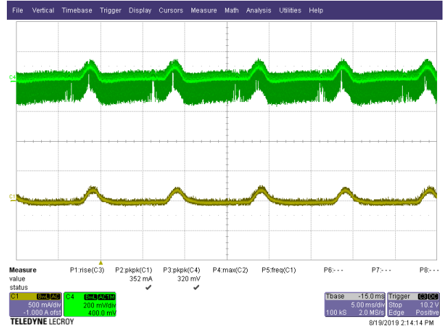
Figure 54 – Output Ripple, 264 VAC, 32 V CV Load. Green: V_{OUT} Ripple, 200 mV / div. Yellow: I_{OUT} Ripple, 500 mA, 5 ms / div.
