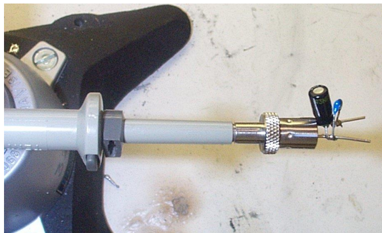
Figure 25 – Oscilloscope Probe with Probe Master ( www.probemaster.com ) 4987A BNC Adapter. (Modified with wires for ripple measurement, and two parallel decoupling capacitors added.)
