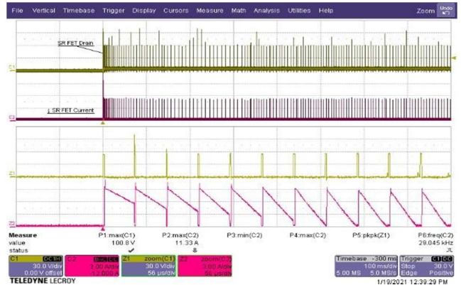
Figure 71 – SR FET Drain Voltage and Current. 265 VAC, 5.0 V, 3 A Load. V_{DS\_SRFET} = 101 V Maximum. CH1: V_{DS\_SRFET} , 30 V / div. CH2: I_{DS\_SRFET} , 3 A / div. Time: 100 ms / div. (56 \mu s / div. Zoom)
