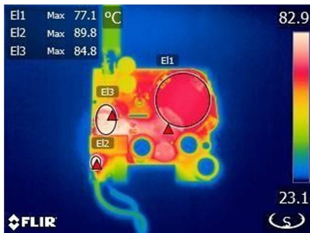
Figure 50 – Top Thermal Image, T_{AMB} = 23.5 °C. E1: Transformer, T_1 = 77.1 °C. E2: Thermistor, RT_1 = 89.8 °C. E3: CMC, L_1 = 84.8 °C.
