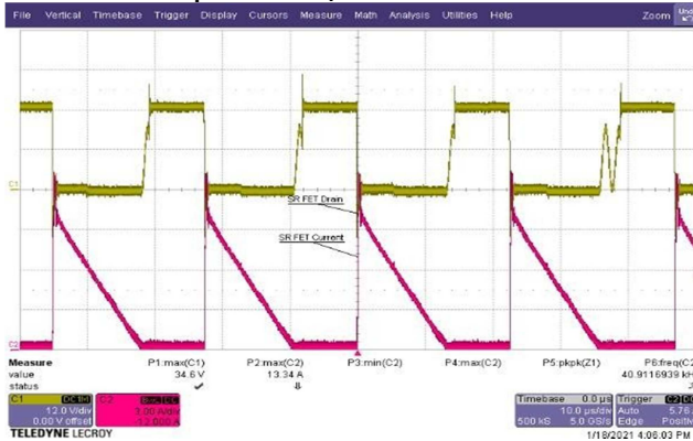
Figure 84 – SR FET Drain Voltage and Current. 90 VAC, 9.0 V, 3 A Load. V_{DS\_SRFET} = 34.6 V Maximum. CH1: V_{DS\_SRFET} , 12 V / div. CH2: I_{DS\_SRFET} , 3 A / div. Time: 10 \mu s / div.
