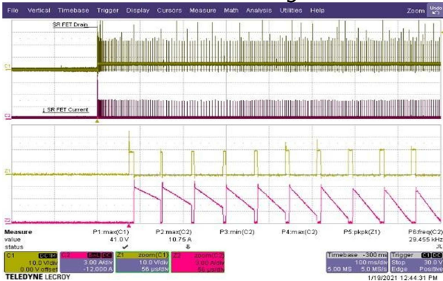
Figure 70 – SR FET Drain Voltage and Current. 90 VAC, 5.0 V, 3 A Load. V_{DS\_SRFET} = 41 V Maximum. CH1: V_{DS\_SRFET} , 10 V / div. CH2: I_{DS\_SRFET} , 3 A / div. Time: 100 ms / div. (56 \mu s / div. Zoom)
