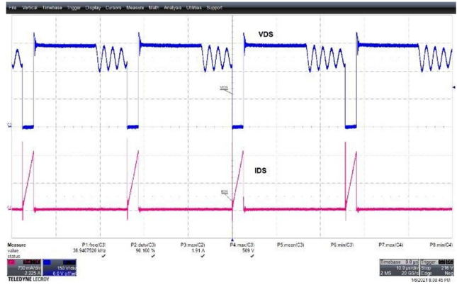
Figure 75 – Primary Drain Voltage and Current. 265 VAC, 9.0 V, 3 A Load. V_{DS\_PRI} = 509 V Maximum. CH1: V_{DS\_PRI} , 150 V / div. CH2: I_{DS\_PRI} , 750 mA / div. Time: 10 \mu s / div.
