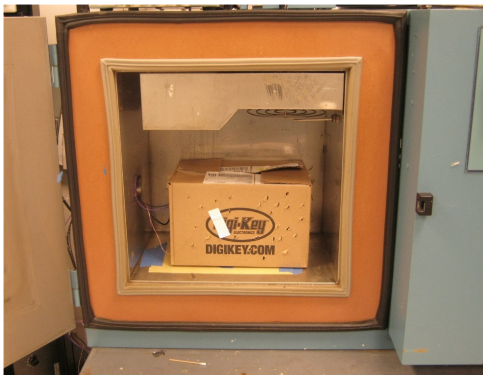
Figure 34 – Isolation Box in Thermal Chamber.
