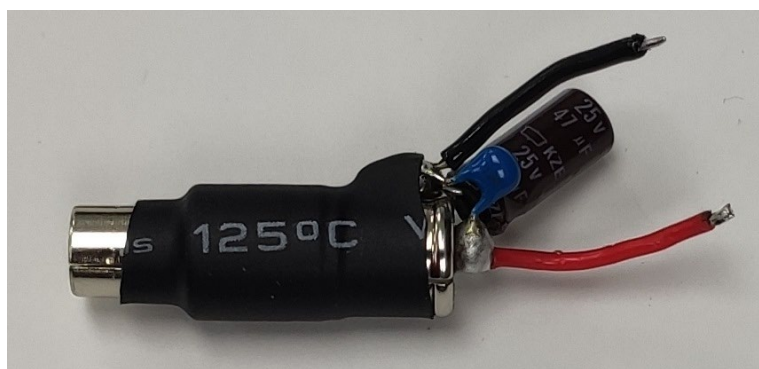
Figure 111 – Probe Master ( www.probemaster.com ) 4987A BNC Adapter. (Modified with wires for ripple measurement, and two parallel decoupling capacitors added.)
