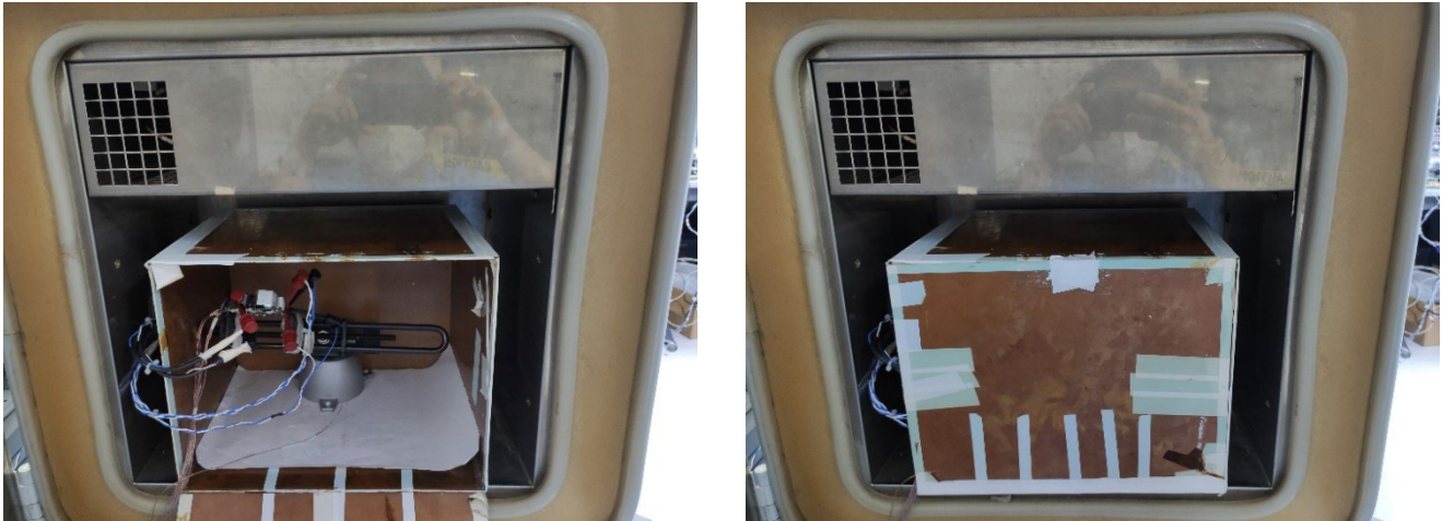
Figure 143 – Thermal Performance Set-up Using Thermal Chamber.
